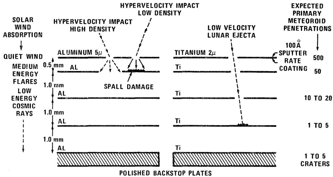
Figure 1. Schematic Illustration of Multiple Foil Lunar Environment Analyser (FLEA) Concept
