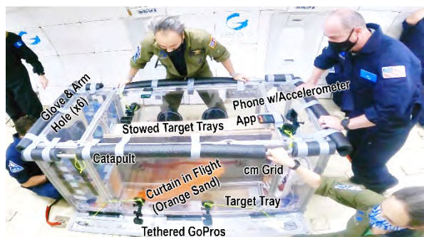
Figure 2. GoPro video still from a Martian gravity (~3.72 m/s 2 ) parabola showing an ejecta curtain and deposit made of green sand being emplaced over prior deposits of blue and orange sand. The just-fired catapult is seen on the left; the two springs are visible behind it. Reflections of personnel are visible in the glovebox sides. GoPro camera lens distortion renders the straight metal sides to appear curved.
