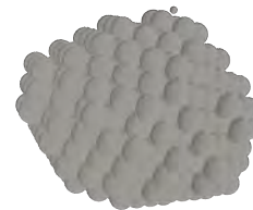
(c) 3D Cartesian, hexagonal close packing, rotated to show impactor height above surface. We again note that these spheres are boulders in a rubble-pile configuration and are not SPH particles.
