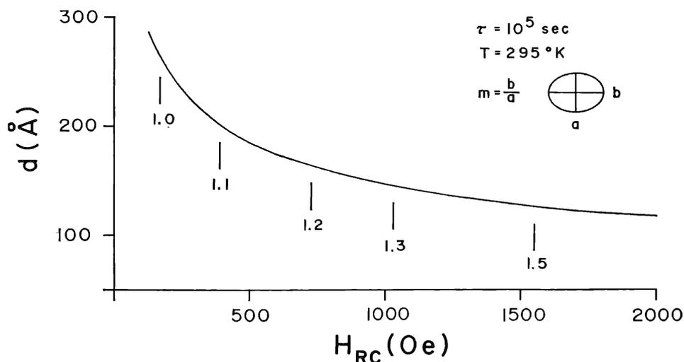
Fig. 2. Dependence of remanent coercivity  $H_{RC}$  on grain size.
