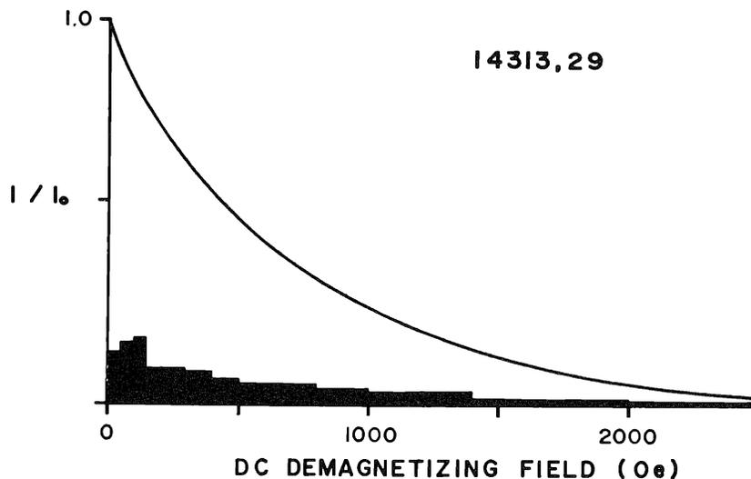
Fig. 3. D.C. demagnetization of IRM acquired in an 18-kilogauss field. Histogram indicates the portion of the intensity removed in a given interval.
