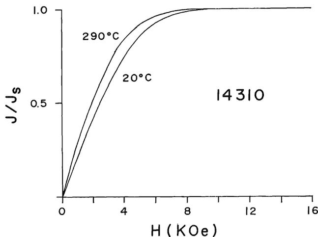
Fig. 6. Magnetization curves for igneous sample 14310 measured at 20°C and 290°C. These curves have been corrected for paramagnetic magnetization and then normalized to  $J_s(T) = 1$ .
