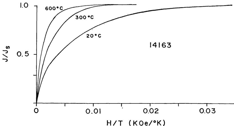
Fig. 8. Magnetization curve for soil with ratio  $H/T$  plotted on abscissa. The magnetization has been corrected for paramagnetic magnetization and then normalized to  $J_s(T) = 1$ .
