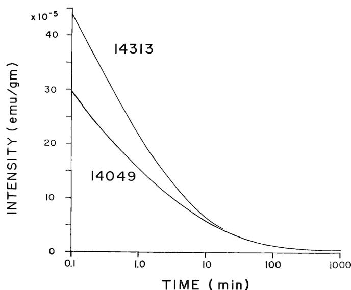
Fig. 1. Decay of VRM induced in samples 14049 and 14313 by a magnetic field of 2.5 Oe. Both samples were measured up to 1000 min.
