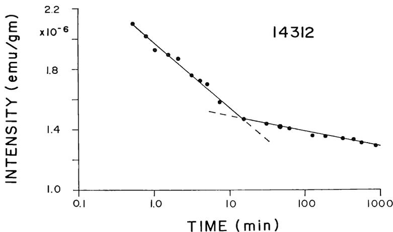
Fig. 5. Decay of VRM induced in sample 14312,7 by a magnetic field of 2.5 Oe.
