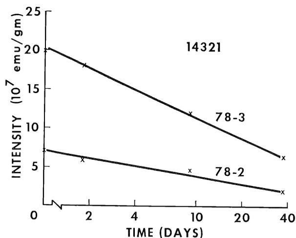
Fig. 4. Decay of natural remanent magnetization of samples 14321,78,2 and 14321,78,3 during storage in a field-free space.
