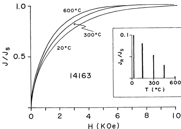
Fig. 7. Magnetization curves for soil 14163 measured at 20°C, 300°C, and 600°C. These curves have been corrected for paramagnetic magnetization and then normalized to  $J_s(T) = 1$ . (Inset) Histogram showing variation of ratio  $J_r/J_s$  with temperature for sample 14163.
