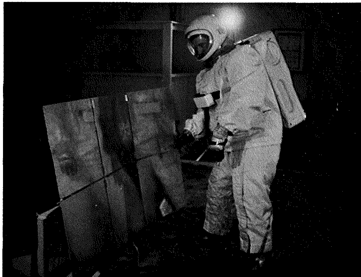
Figure #8 - Subject near completion of deployment of one-half of the solar cell array.
